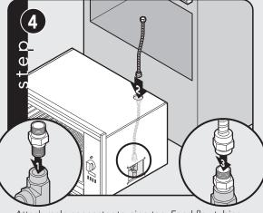
Attach male connector to pipe tee. Feed flex tubing through 2" hole and attach to the male connector.
